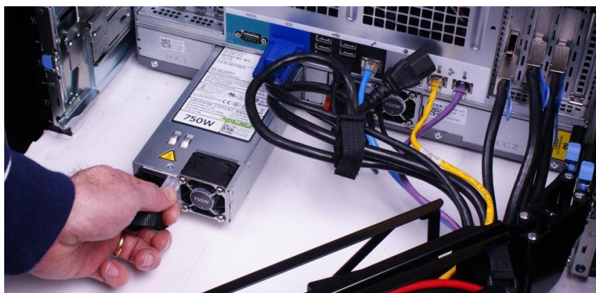
Figure 6. Replacing the power supply
