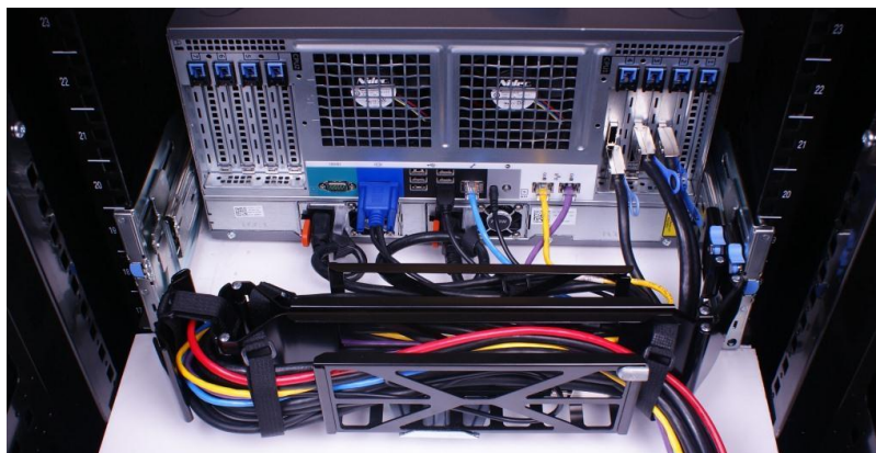
Figure 5. Right-side mounted CMA installation
