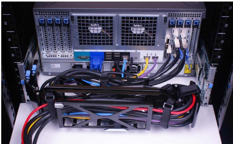
Figure 5. Right-side mounted CMA installation
