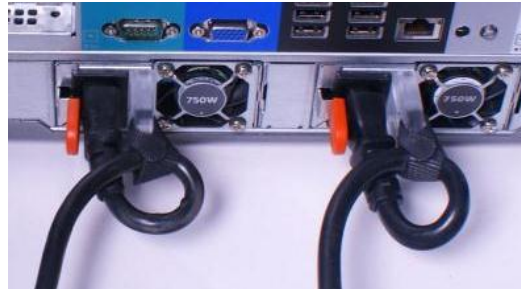
Figure 2. Routing power cables through the strain reliefs
